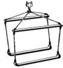
Figure 4-16. Pallet bridle spreaders
