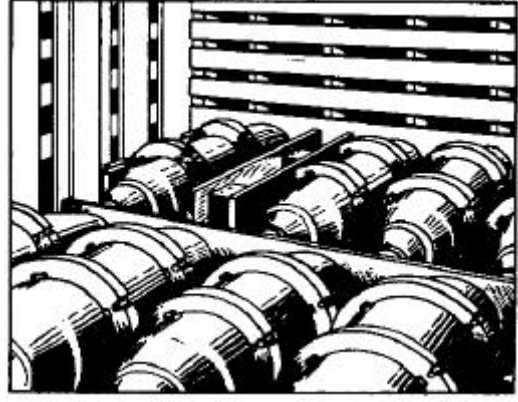
Figure 9-11. Dunnage used to separate bombs
